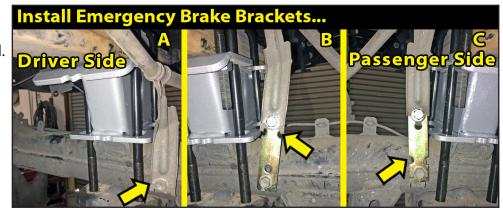
brake bracket using the supplied 5/16" x 3/4" bolt, washers, and Nyloc {1/2"}
