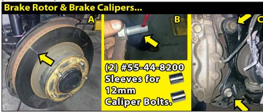
brake caliper onto knuckle and tighten {17mm or 19mm}
