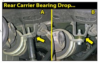
**NOTE:** This is a starting point of adjustment for driveshaft vibration. If you have a vibration during acceleration, make adjustments by adding or removing spacers. Adjust as needed, but always make even adjustments to both sides. [Illustration 46]
